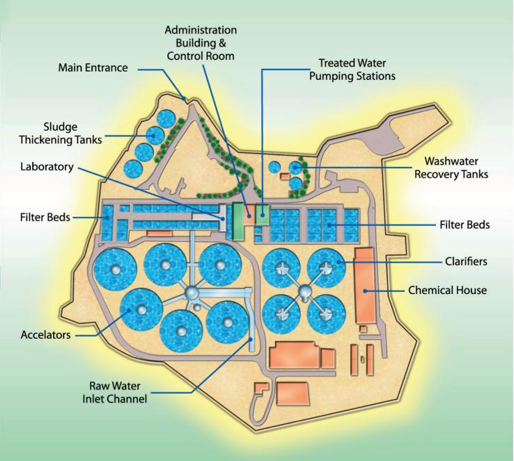
SHA TIN Water Treatment Works is the largest water treatment works in Hong Kong in terms of daily output capacity. It provides treated water supplies to Sha Tin, Central Kowloon and part of Hong Kong Island. It was first commissioned in May 1964 with a treated water output of 364,000 m³/day. It was then extended in stages and the nominal capacity has become 1,227,000 m³/day since 1983.
