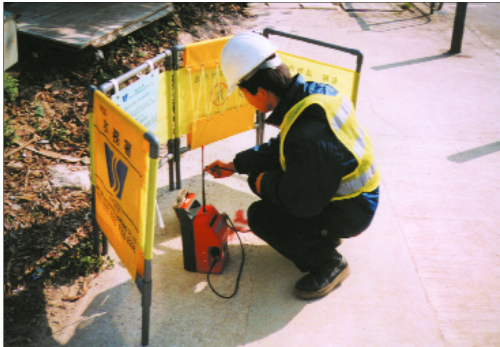
水務署採用最新的聲納探測儀器測漏。 The latest acoustic equipment is used for leak detection.
