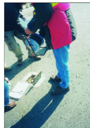
檢視一部設於萬宜水庫西壩頂部的新壓力計。 Inspecting a new piezometer at the High Island West Dam crest.
