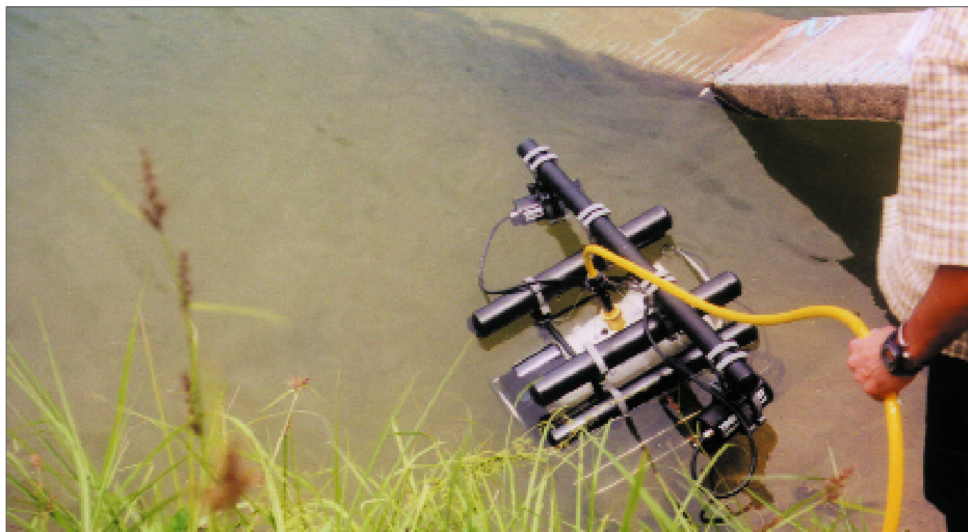
利用一部水底錄影系統檢查堤壩。 An underwater video system is being deployed for dam inspection.
