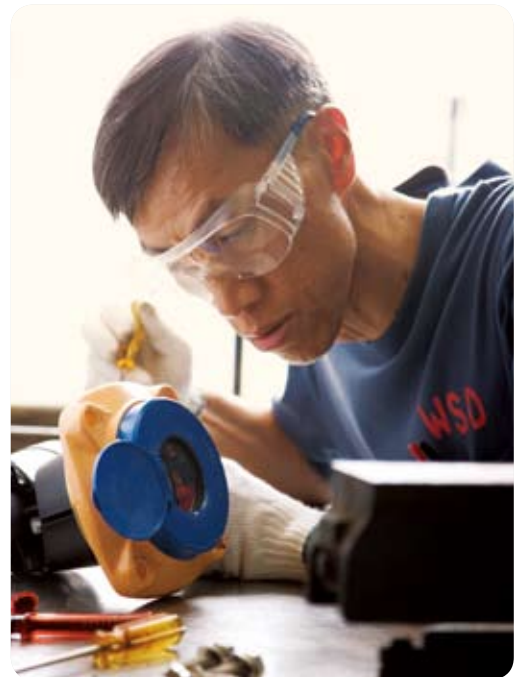
水務設施條例規定，水錶的偏差程度不可超出±3%，而這亦是本署向客戶承諾的整體水錶準確程度表現目標。 The Waterworks Regulations stipulate inaccuracy of water meters should not exceed ±3%. This is also the performance target on the overall meter accuracy pledged by the Department to customers.
