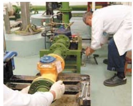
測試大型水錶的準確程度。 Conducting accuracy test on a large water meter.
