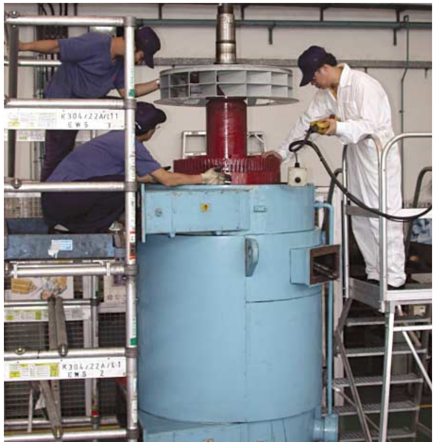
技術人員於電機工場內維修一座大型電動機。 A large electric motor being overhauled in Electrical Workshop.
