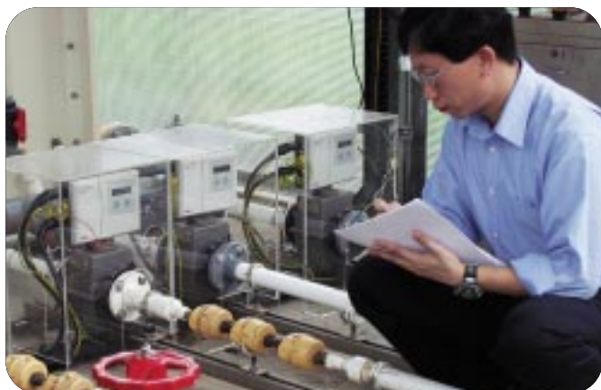
正進行水錶加速損耗的測試。 Conducting water meter accelerated wear test.
