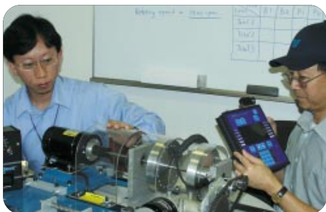
利用先進儀器監察電動機和水泵的振動情況。 Using state-of-the-art equipment to monitor electric motor and pump vibration.
