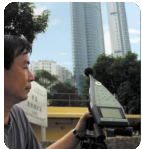
定期測試抽水站發出的噪音水平，確保符合噪音管制的規定。 Regular testing of sound level of pumping stations to ensure compliance of noise emission requirement.
