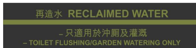
Figure 8-5 Recommended Labelling for Reclaimed Water Pipes Located Outside Buildings or Below Ground
