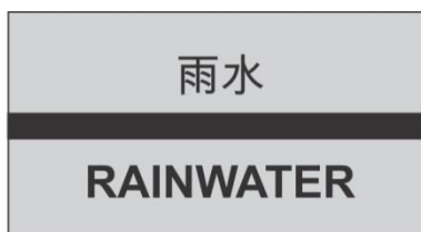
Figure 8-1 Example of Labelling for Rainwater Collection Pipes
