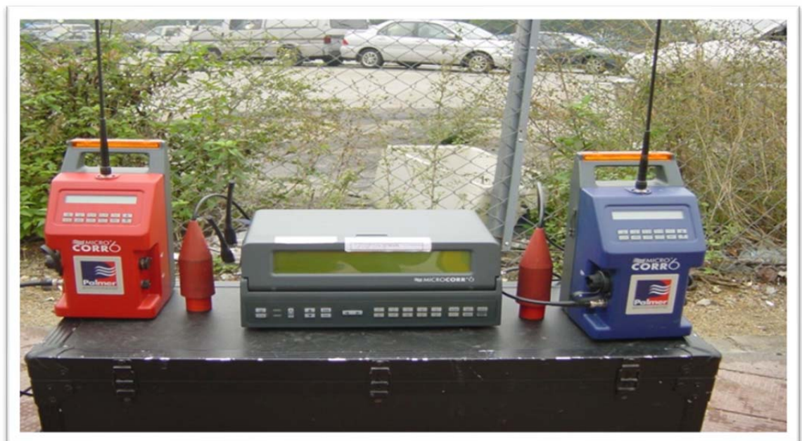
Photo 3 Equipment for leak noise detection
