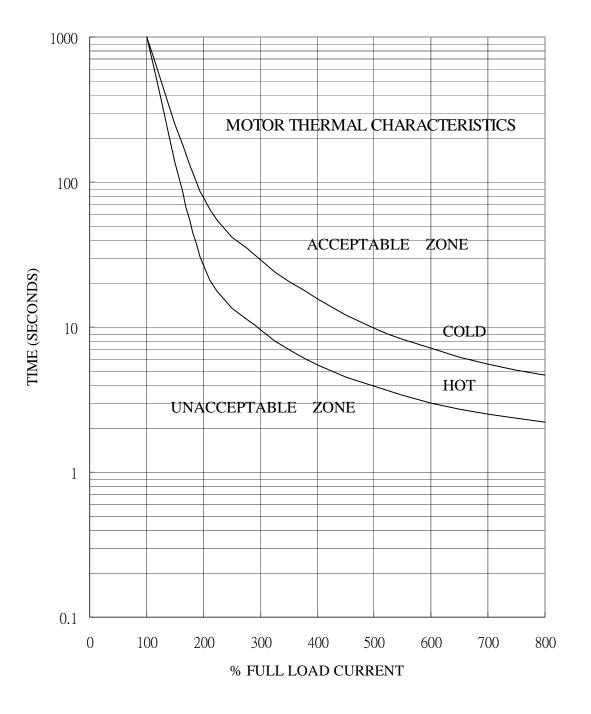
Motor Short-time Overload Withstand Characteristics
