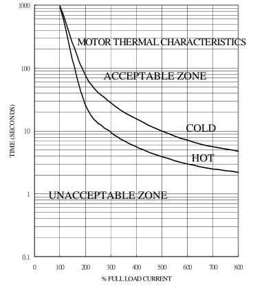
Motor Short-time Overload Withstand Characteristic
