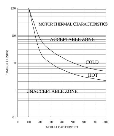
**Motor Short-time Overload Withstand Characteristics**
