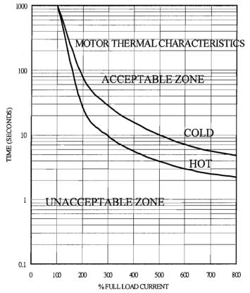
**Motor Short-time Overload Withstand Characteristic**
