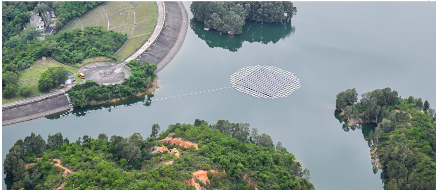
大欖涌水塘的浮動太陽能板發電系統 Floating PV System at Tai Lam Chung Reservoir
