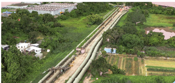
透過無人機攝影測量法獲取的點雲記錄 Point cloud records taken by unmanned aerial vehicle photogrammetry.
