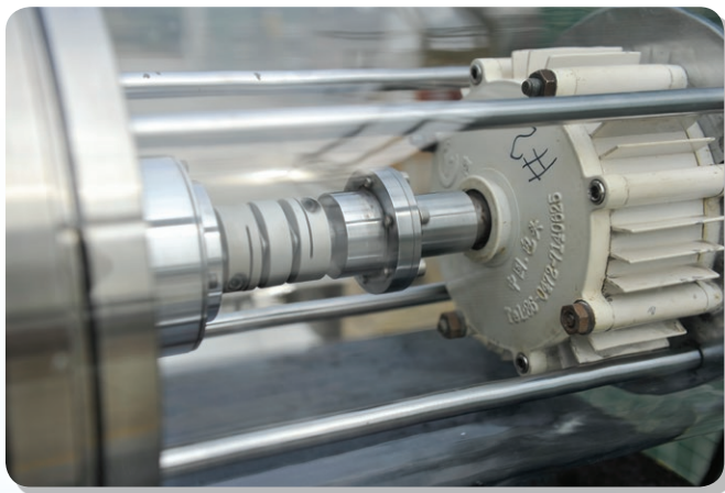
內聯閉式水力發電系統的模型。 The model of inline hydroelectric generating system in confined condition.
