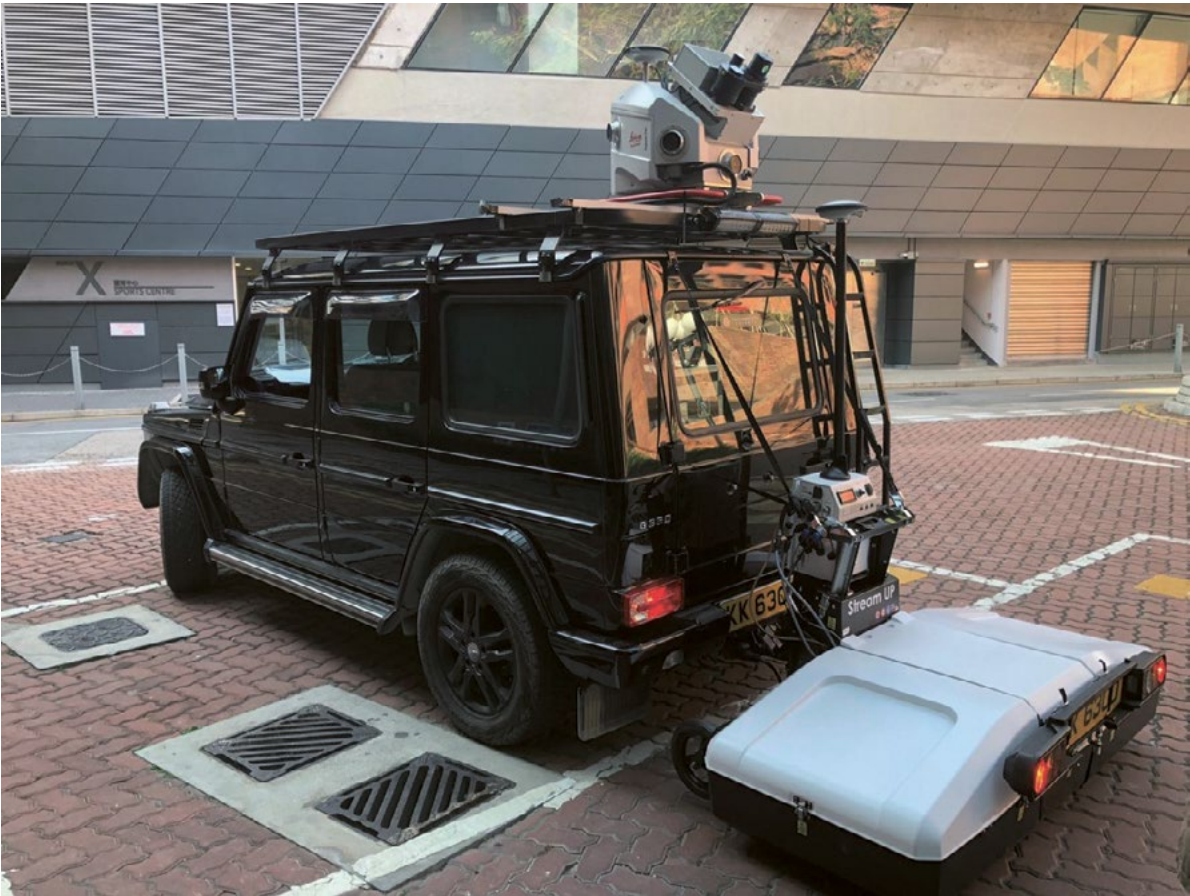
▲ Investigation of groundwater pipes using GPR
