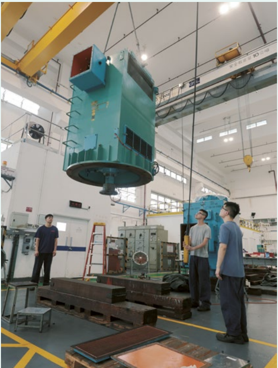
▲ The electrical workshop is equipped with a large crane to facilitate the movement of motors.
