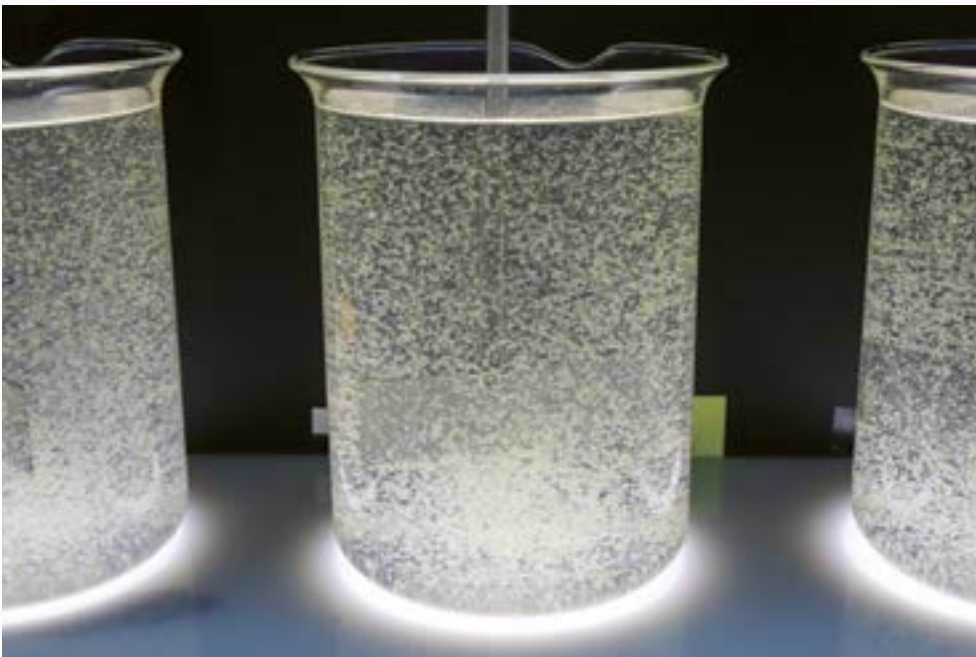
▲ Alum causes the suspended impurities in the raw water to coagulate and flocculate into larger particles.
