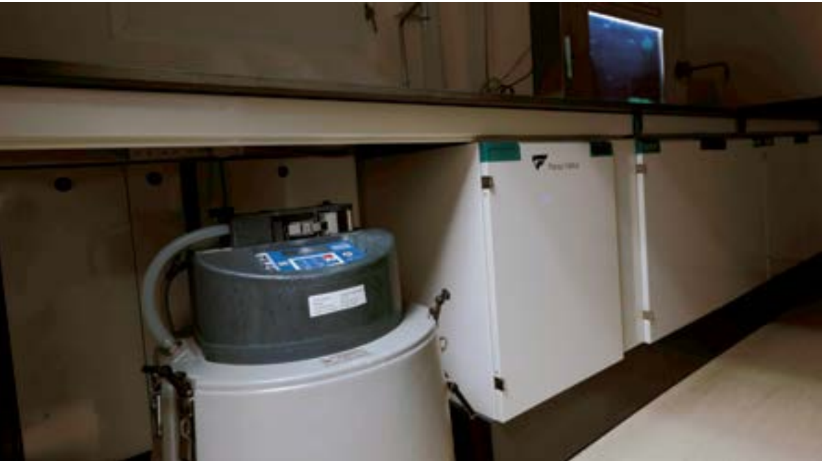
▲ The Sheung Shui Water Treatment Works is the first water treatment works to adopt the Biosensing Alert System. When a zebrafish behaves abnormally, the alert system will sound an alarm and automatically take water samples for testing. The bottom left corner of the picture shows the sampler.
