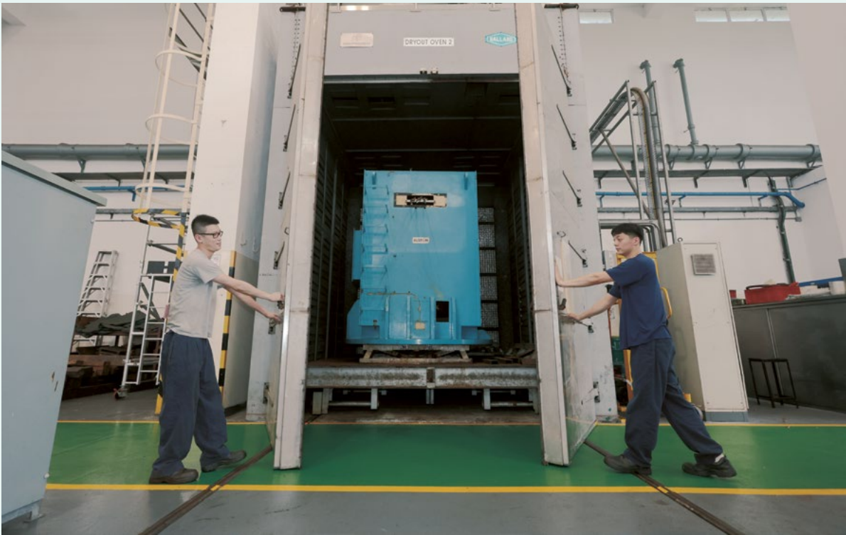
▲ The motor workshop is equipped with a large motor baking oven to extract moisture from a motor to ensure its insulation.
