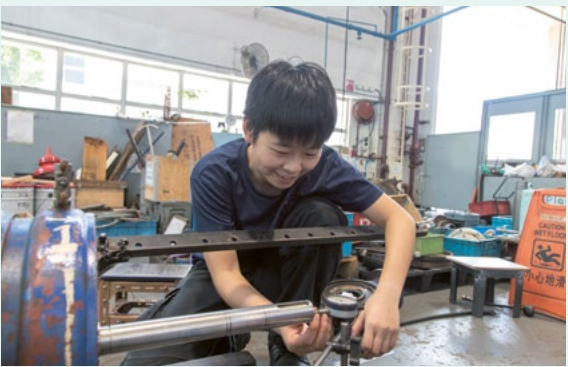
▲ An apprentice adjusts the position of the impellers of a multi-layer pump ensuring that each impeller is in the middle of the pump to maintain maximum pump efficiency.
