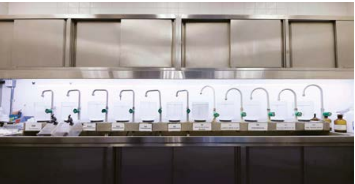
▲ The control room of the water treatment works has various "clarify bowls", for easy inspection by operators analysing the condition of the water samples after the completion of each treatment process.
