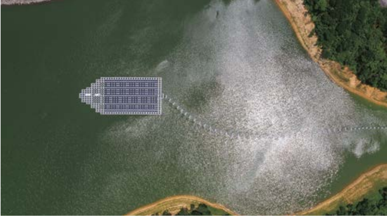
▲ The floating solar power system at the Plover Cove Reservoir has solar PV panels shaped like a boat.
